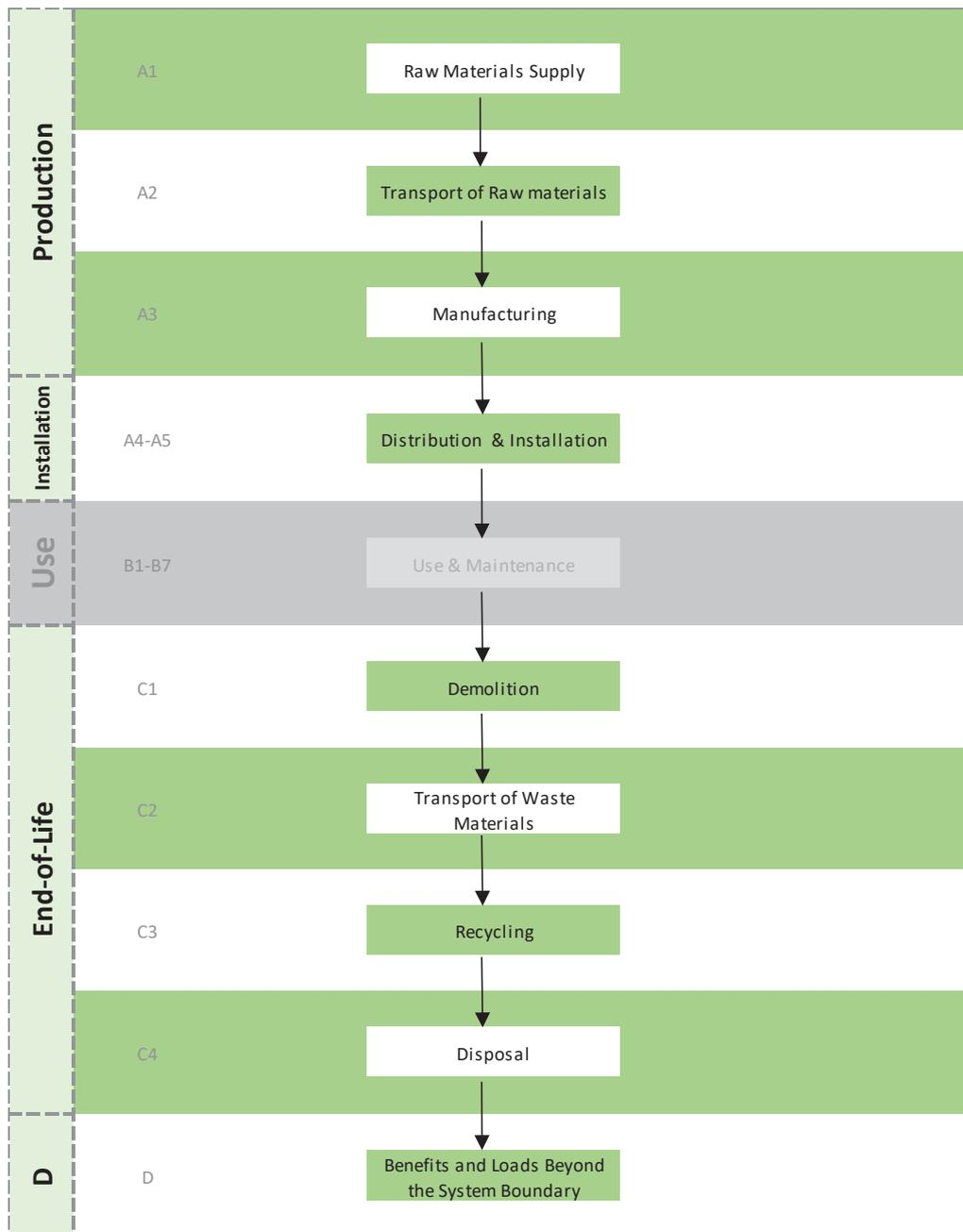
Figure 1. System diagram for the life cycle of the fabric
