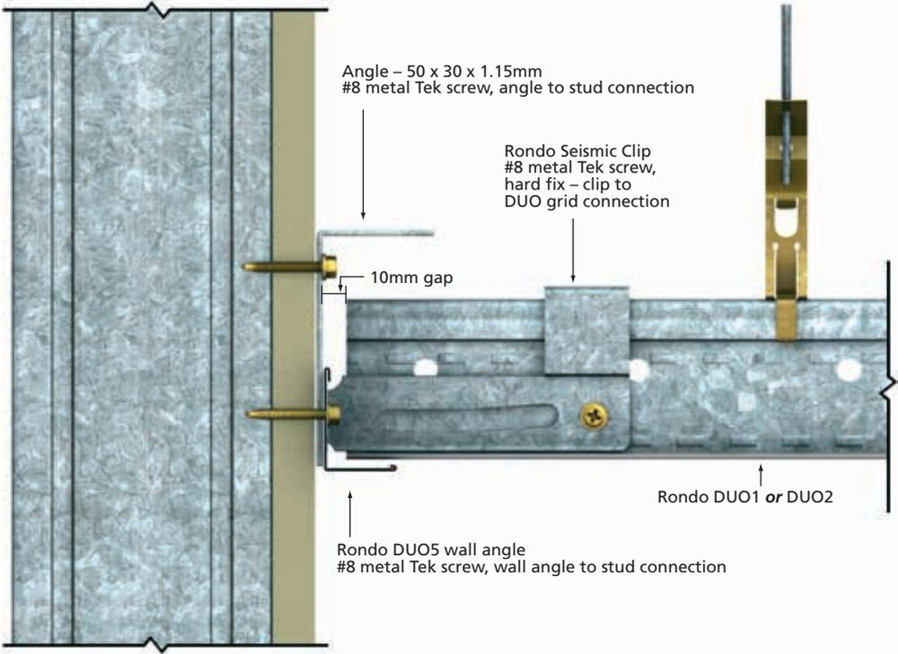
● DUO GRID FIXING TO STUDWALL — FIXED CONNECTION
