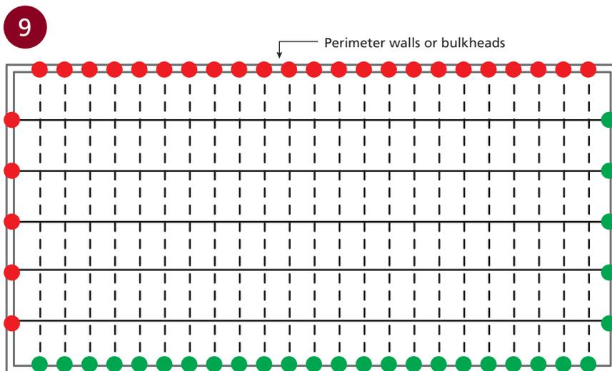
■ DUO® CEILING PLAN – TYPICAL PERIMETER FIXING ARRANGEMENT
