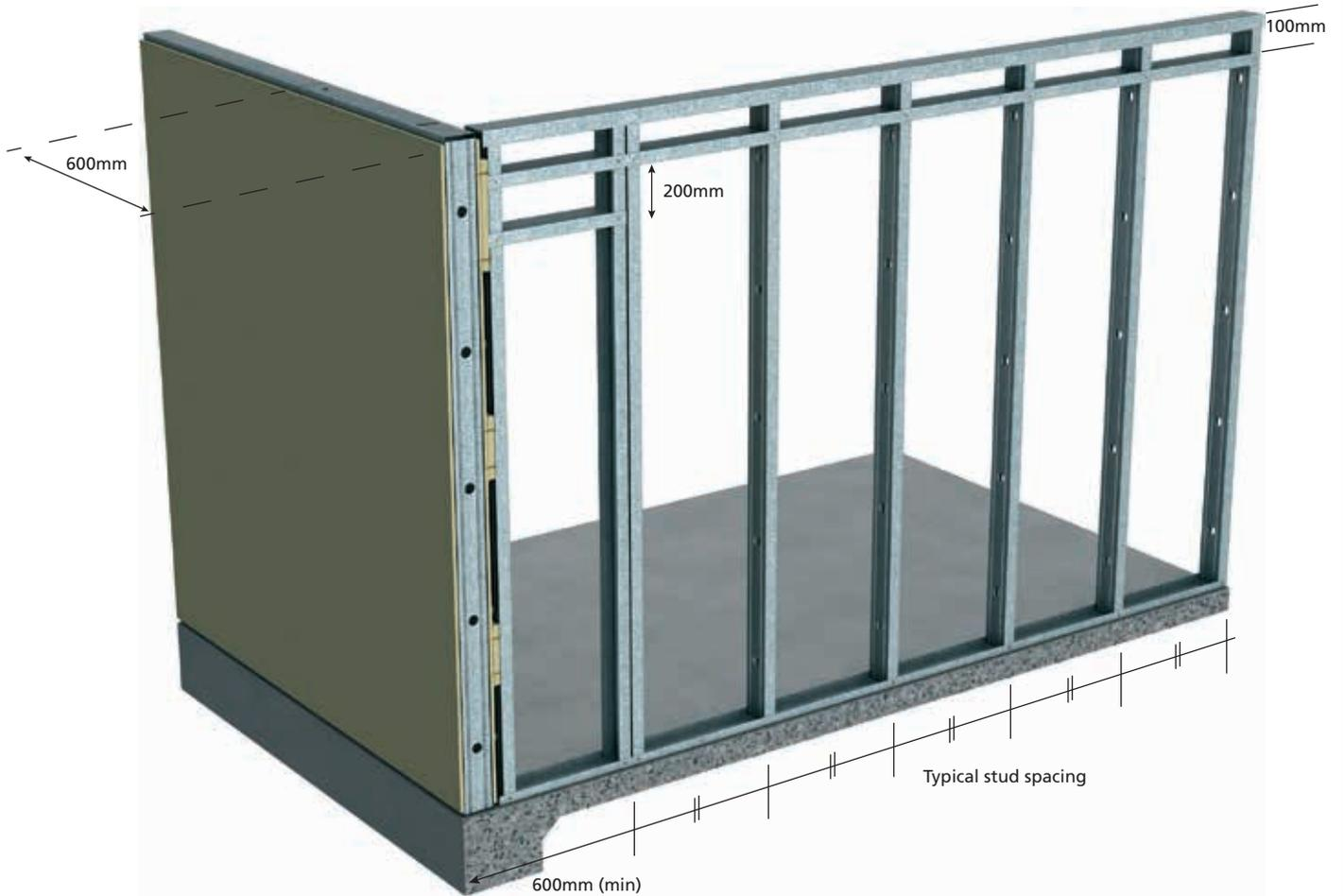
NOTE: This is a pictorial only, a midspan nogging may be required depending on wall height and lining conditions, refer to the Rondo Professional Design Manual for nogging requirements.
