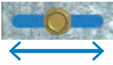
Indicates the fixing slot in the Rondo Seismic Slotted Deflection Head Track. The slot allows displacement of adjacent Wall Studs, letting them slide within the Tracks in the direction shown by the arrows. The movement occurs at the head whilst the wall framing is stabilised at the base.
