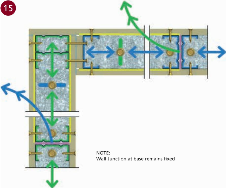
■ STUD WALL ARTICULATION/MOVEMENT AT CORNER JUNCTION AT HEAD
