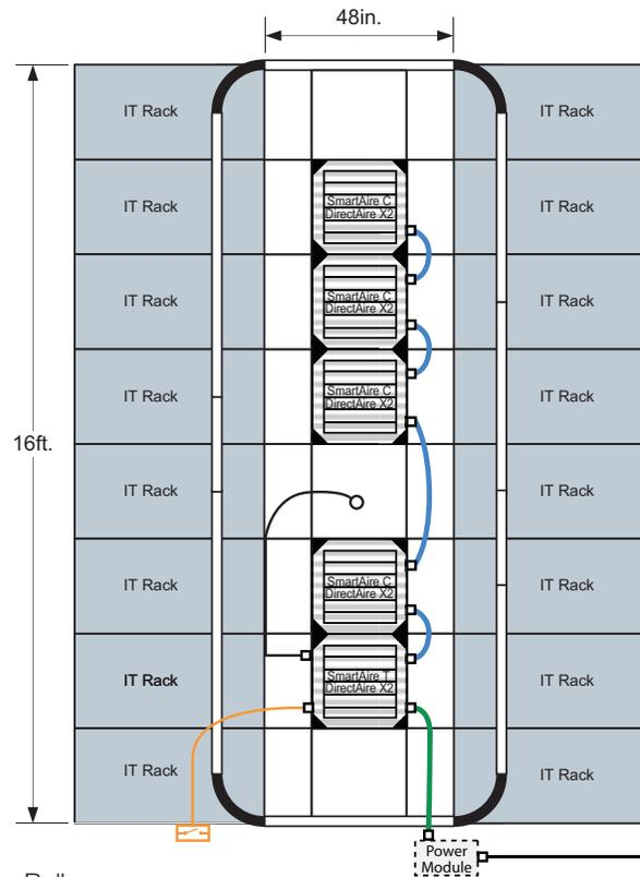
The user would be required to provide the hot aisle entrance signal, in this case a latching entrance switch has been chosen to signal to the SmartAire T to begin temperature control of the hot aisle.
