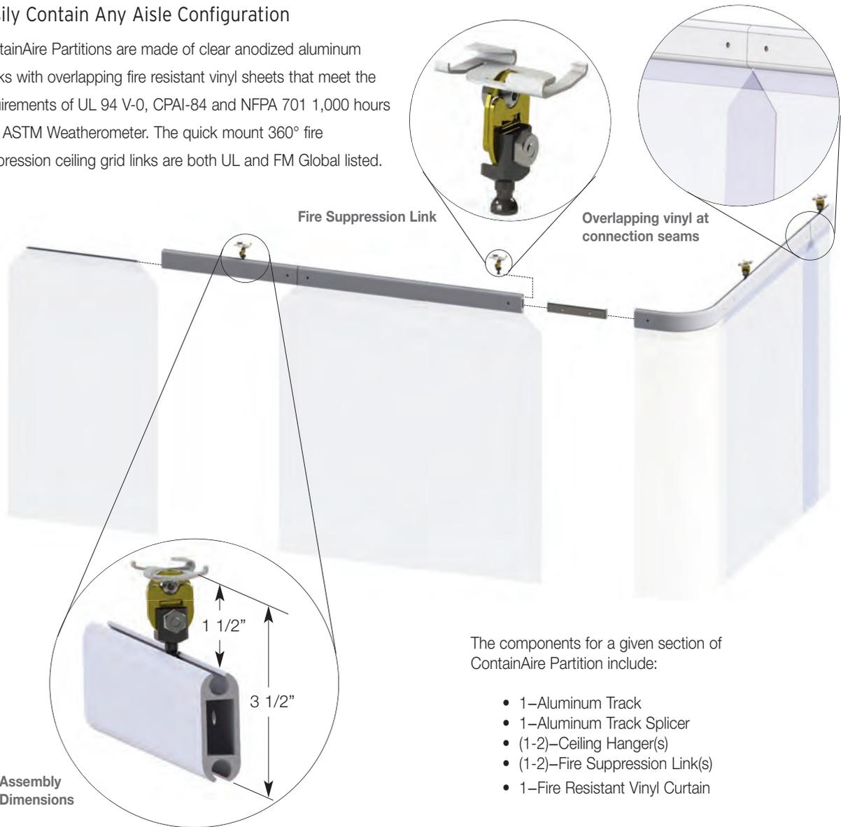
The components for a given section of ContainAire Partition include:
